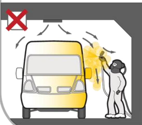
FIGURE 7 The operator is exposed to overspray and reaching above shoulder height can cause discomfort and injury to the body
