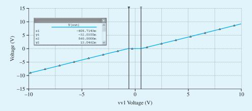
Figure B.106 VTC of class B output stage.
