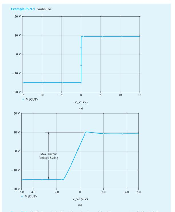
Figure B.27 (a) The large-signal differential transfer characteristic of the op-amp circuit in Fig. B.26. The common-mode input voltage  $V_{CM}$  is set to 0 V. (b) An expanded view of the transfer characteristic in the high-gain region.
