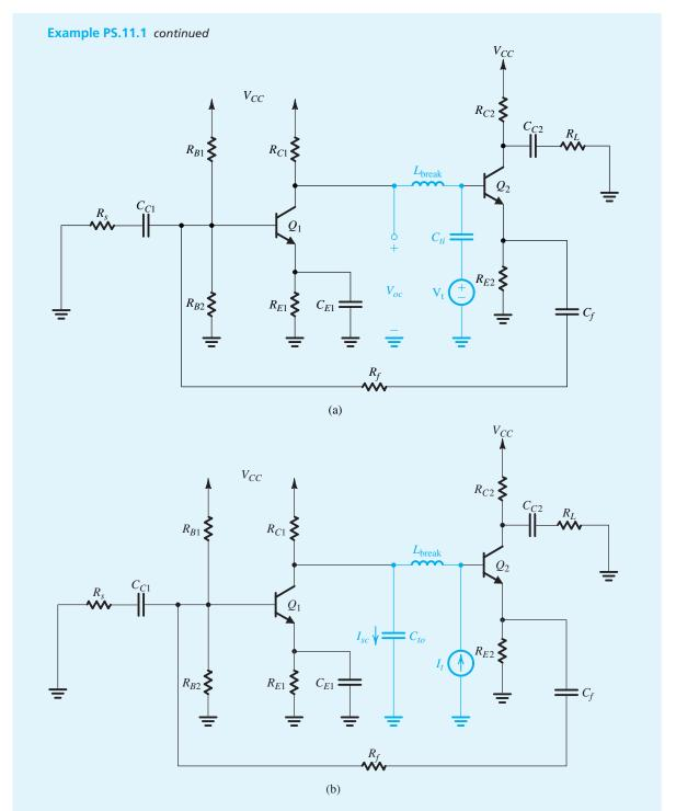
**Figure B.34** Circuits for simulating (a) the open-circuit voltage transfer function  $T_{oc}$  and (b) the short-circuit current transfer function  $T_{gc}$  of the feedback amplifier in Fig. B.33 for the purpose of computing its loop gain.
