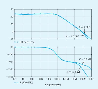
**Figure B.46** Magnitude and phase response of the op-amp circuit in Fig. B.43:  $C_c = 0.6 \text{ pF}$ ,  $R = 1.53 \text{ k}\Omega$  ( $PM = 55^\circ$ ), and  $R = 3.2 \text{ k}\Omega \ (PM = 75^{\circ}).$
