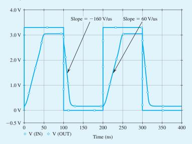
**Figure B.48** Large-signal step response (for a 3.3-V step-input) of the op-amp circuit in Fig. B.43 connected in a unity-gain configuration. The slope of the rising and falling edges of the output waveform correspond to the slew rate of the op amp.
