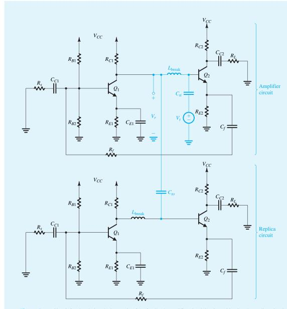
Figure B.35 Circuit for simulating the loop gain of the feedback amplifier circuit in Fig. B.33 using the replica-circuit method.
