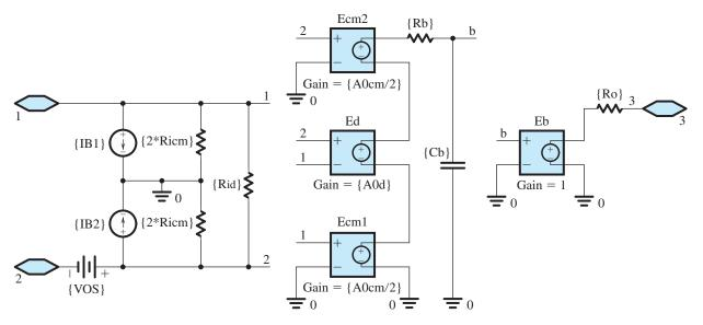
Figure B.2 A comprehensive linear macromodel of an internally compensated op amp.
