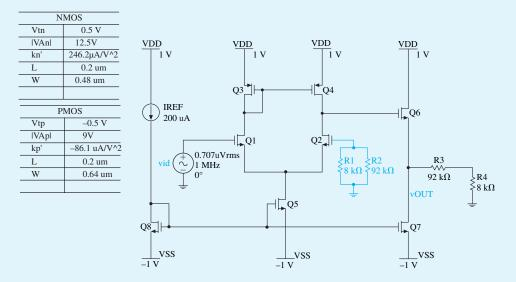
**Figure B.98** Schematic capture of the *A*-circuit.
