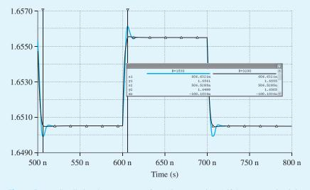
**Figure B.112** Small-signal step response (for a 10-mV step input) if the op-amp circuit is connected in a unity-gain configuration:  $PM = 55^{\circ}$  ( $C_C = 0.6$  pF, R = 1.53 k $\Omega$ ) and  $PM = 75^{\circ}$  ( $C_C = 0.6$  pF, R = 3.2 k $\Omega$ ).
