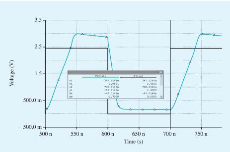
Figure B.113 Large-signal step response (for a 2.2-V step input) if the op-amp circuit is connected in a unity-gain configuration. The slope of the rising and falling edges of the output waveform correspond to the slew rate of the op amp.
