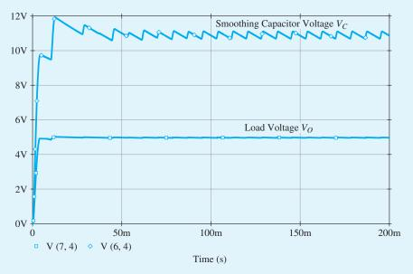
Figure B.14 The voltage  $v_{\hat{o}}$  across the smoothing capacitor C and the voltage  $v_{\hat{o}}$  across the load resistor  $R_{\text{load}} = 200 \,\Omega$  in the 5-V power supply of Example PS.4.1.
