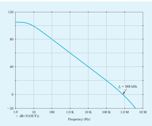
**Figure B.10** Frequency response of the μA741 op amp in Example PS.2.2.
