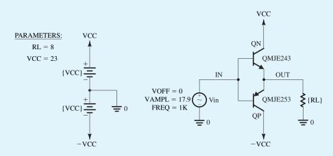
**Figure B.37** Capture schematic of the class B output stage in Example PS.12.1.
