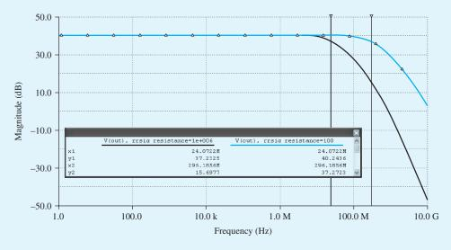
**Figure B.94** Frequency response of the folded-cascode amplifier with  $R_{\text{sig}} = 100 \, \Omega$  and  $R_{\text{sig}} = 1 \, \text{M}\Omega$ .
