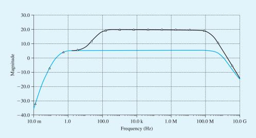
Figure B.90 Frequency response of the CS amplifier with  $C_s = 10 \,\mu\text{F}$  and  $C_s = 0$ .
