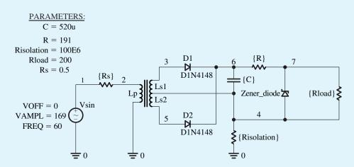
**Figure B.13** Schematic capture of the 5-V dc power supply in Example PS.4.1.
