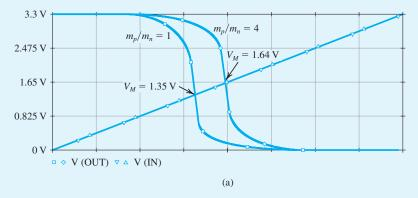
Figure B.51 (a) Output voltage and (b) supply current versus input voltage for the CMOS inverter in Example PS.14.1 with  $m_n/m_n = 1$  and  $m_n/m_n = 4$ .
