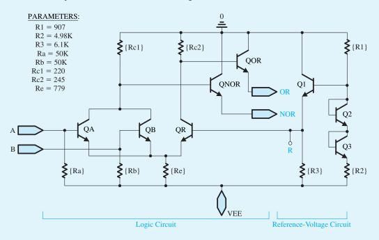
Figure B.53 Schematic capture of the two-input ECL gate for Example PS.15.1
