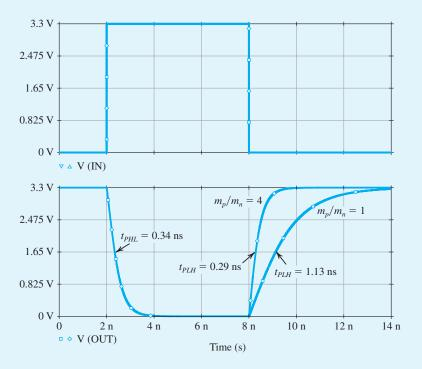
Figure B.52 Transient response of the CMOS inverter in Example PS.13.1 with  $m_p/m_p = 1$  and  $m_p/m_p = 4$ .
