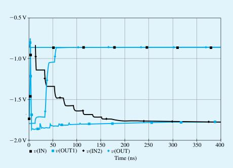
Figure B.59 Transient response of a cascade of two ECL gates interconnected by a 1.5-m cable having a characteristic impedance of  $300 \Omega$ . The termination resistance  $R_{T1}$  (see Fig. B.57) was kept unchanged at  $50 \Omega$ . Note the change in time scale of the plot.
