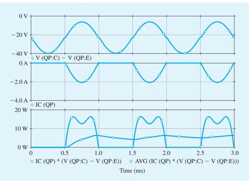
Figure B.40 Waveforms of the voltage across, the current through, and the power dissipated in the pnp transistor  $Q_p$ of the output stage shown in Fig. B.37.
