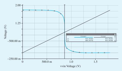
Figure B.117 Output voltage versus input voltage for the inverter (to the threshold voltage measure  $V_{i}$ ).
