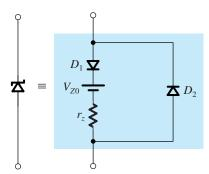
Figure B.4 Equivalent-circuit model used to simulate the zener diode in SPICE. Diode  $D_1$  is ideal and can be approximated in SPICE by using a very small value for n (say
