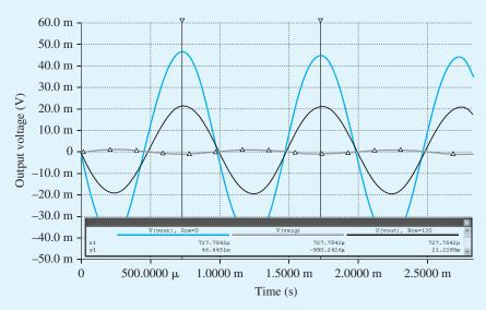
**Figure B.76** Transient analysis of the CE amplifier with  $R_{ce} = 0$  and  $R_{ce} = 130 \Omega$ .
