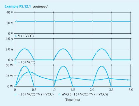
**Figure B.39** The voltage (upper graph), current (middle graph), and instantaneous and average power (bottom graph) supplied by the positive voltage supply  $(+V_{CC})$  in the circuit of Fig. B.37.
