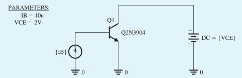
Figure B.19 The PSpice test bench used to demonstrate the dependence of  $\beta_{de}$  on the collector bias current  $I_c$  for the Q2N3904 discrete BJT (Example PS.6.1).
