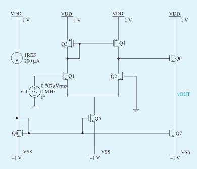
Figure B.95 Schematic capture of the two-stage CMOS op amp.
