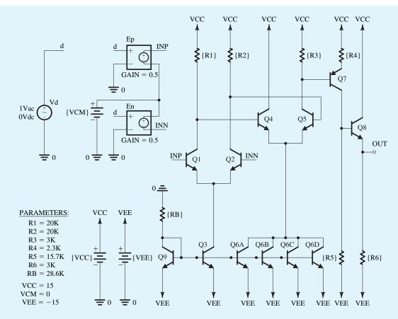
**Figure B.26** Schematic capture of the op-amp circuit in Example 7.6.
