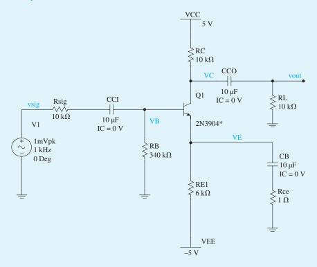
Figure B.75 Schematic capture of the CE amplifier.
