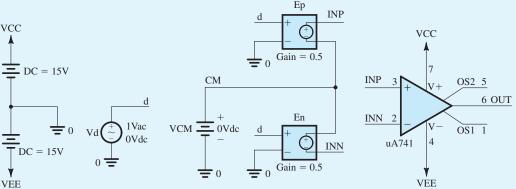
Figure B.9 Simulating the frequency response of the μA741 op-amp in Example PS.2.2.
