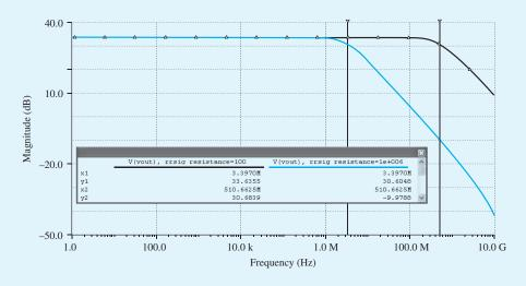
**Figure B.92** Frequency response of the CMOS CS amplifier with  $R_{\text{sig}} = 100 \,\Omega$  and  $R_{\text{sig}} = 1 \,\text{M}\Omega$ .
