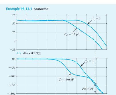
**Figure B.44** Magnitude and phase response of the op-amp circuit in Fig. B.43:  $R=1.53~\mathrm{k}\Omega$ ,  $C_{c}=0$  (no frequency compensation), and  $C_{c}=0.6~\mathrm{pF}$  ( $PM=55^{\circ}$ ).
