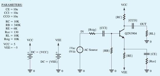
Figure B.21 Schematic capture of the CE amplifier in Example PS.7.2.
