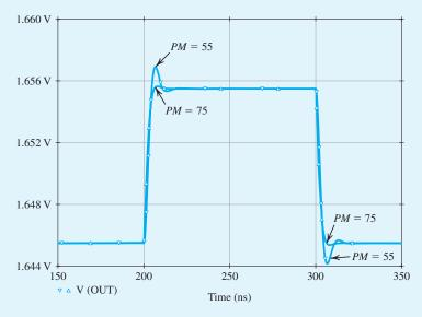
**Figure B.47** Small-signal step response (for a 10-mV step input) of the op-amp circuit in Fig. B.43 connected in a unity-gain configuration:  $PM = 55^{\circ}$  ( $C_C = 0.6$  pF, R = 1.53 k $\Omega$ ) and  $PM = 75^{\circ}$  ( $C_C = 0.6$  pF, R = 3.2 k $\Omega$ ).
