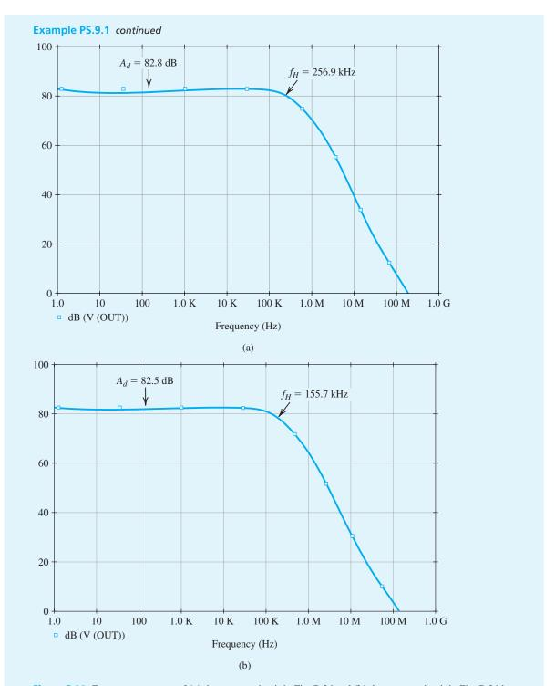
**Figure B.28** Frequency response of (a) the op-amp circuit in Fig. B.26 and (b) the op-amp circuit in Fig. B.26 but with a resistor  $R'_3 = R_3$  inserted in the collector of  $Q_4$  to make the op-amp circuit symmetrical.
