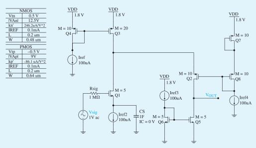
Figure B.93 Schematic capture of the folded-cascode amplifier.
