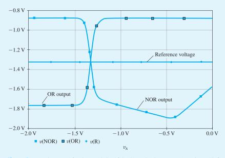
Figure B.55 Voltage transfer characteristics of the OR and NOR outputs (see Fig. B.54) for the ECL gate shown in Fig. B.53. Also indicated is the reference voltage,  $V_{R} = -1.32 \text{ V}$ .
