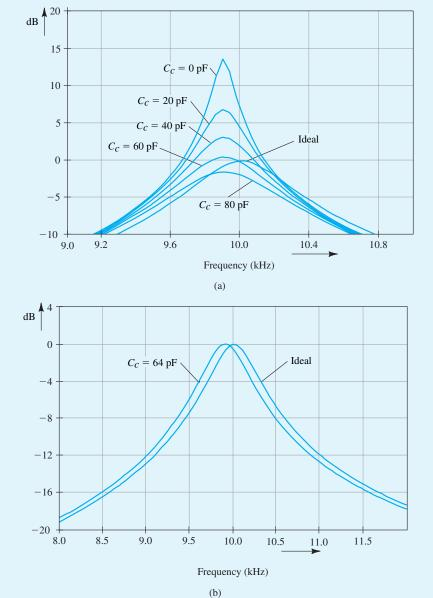
**Figure B.65** (a) Magnitude response of the Tow–Thomas biquad circuit with different values of compensation capacitance. For comparison, the ideal response is also shown. (b) Comparing the magnitude response of the Tow–Thomas biquad circuit using a 64-pF compensation capacitor and the ideal response.
