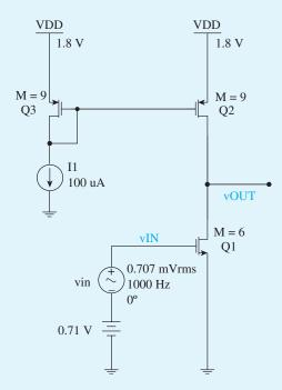
Figure B.78 Schematic capture of the CMOS CS amplifier.
