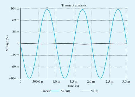
**Figure B.83**  $G_n$  of the folded-cascode amplifier (transient analysis).
