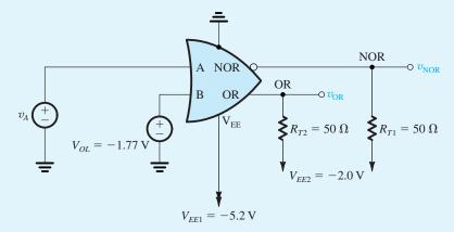
Figure B.54 Circuit arrangement for computing the voltage transfer characteristics of the ECL gate in Fig. B.53.
