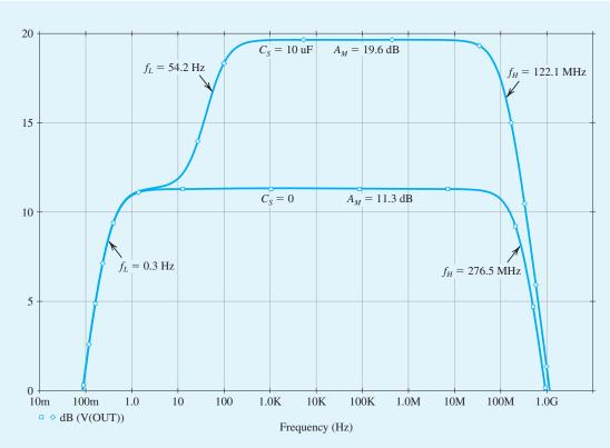
Figure B.18 Frequency response of the CS amplifier in Example PS.7.1 with  $C_S = 10 \,\mu\text{F}$  and  $C_S = 0$  (i.e.,  $C_S$ removed).
