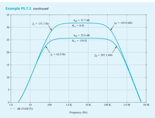
**Figure B.22** Frequency response of the CE amplifier in Example PS.7.3 with  $R_{cc} = 0$  and  $R_{cc} = 130 \Omega$ .
