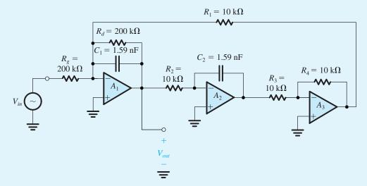
**Figure B.63** Circuit for Example PS.17.2 Second-order bandpass filter implemented with a Tow-Thomas biquad circuit having  $f_0 = 10 \, \text{kHz}$ , Q = 20, and unity center-frequency gain.
