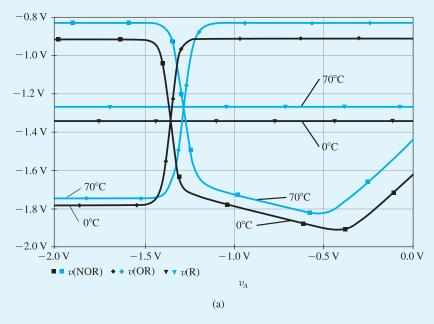
**Figure B.56** Comparing the voltage transfer characteristics of the OR and NOR outputs (see Fig. B.54) of the ECL gate shown in Fig. B.53, with the reference voltage  $V_R$  generated using: (a) the temperature-compensated bias network of Fig. B.53; (b) a temperature-independent voltage source.
