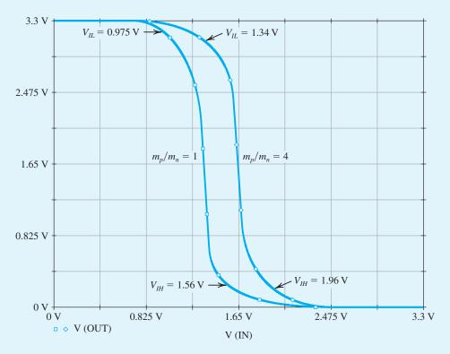
Figure B.50 Input-output voltage transfer characteristic (VTC) of the CMOS inverter in Example PS.14.1 with  $m_{n}/m_{n} = 1$  and  $m_{n}/m_{n} = 4$ .
