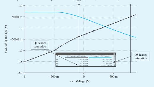
Figure B.85 Input common—mode range of the two-stage CMOS op amp.
