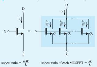
Figure B.24 Transistor equivalency.
