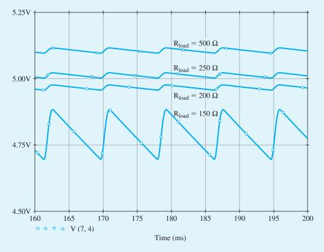
**Figure B.15** The output-voltage waveform from the 5-V power supply (in Example PS.4.1) for various load resistances:  $R_{\text{load}} = 500 \,\Omega$ ,  $250 \,\Omega$ ,  $200 \,\Omega$ , and  $150 \,\Omega$ . The voltage regulation is lost at a load resistance of  $150 \,\Omega$ .
