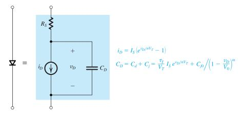
Figure B.3 The SPICE diode model.
