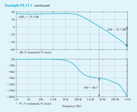
**Figure B.36** (a) Magnitude and (b) phase of the loop gain  $A\beta$  of the feedback amplifier circuit in Fig. B.33.
