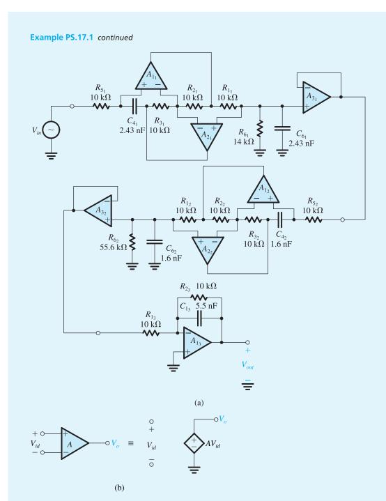
**Figure B.60** Circuits for Example PS.17.1. (a) Fifth-order Chebyshev filter circuit implemented as a cascade of two second-order simulated LCR resonator circuits and a single first-order op amp–RC circuit. (b) VCVS representation of an ideal op amp with gain A.
