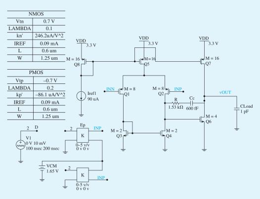
Figure B.108 Schematic capture of the two-stage CMOS op amp.
