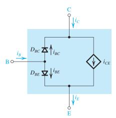
**Figure B.5** The transport form of the Ebers–Moll model for an *npn* BJT.
