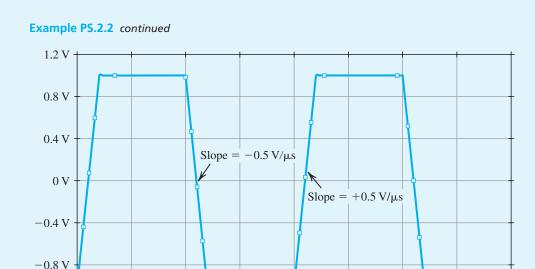
Figure B.12 Square-wave response of the  $\mu$ A741 op amp connected in the unity-gain configuration shown in Fig. B.11.
