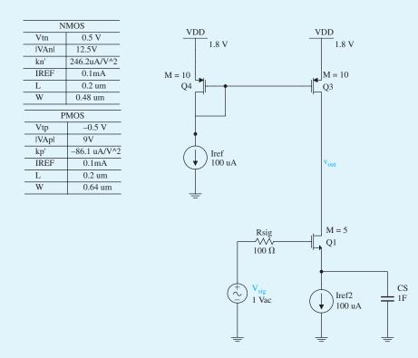
Figure B.91 Schematic capture of the CMOS CS amplifier.
