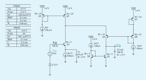
Figure B.82 Schematic capture of the folded-cascode amplifier.
