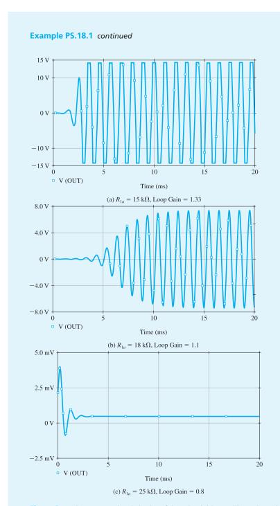
**Figure B.67** Start-up transient behavior of the Wien-bridge oscillator shown in Fig. B.66 for various values of loop gain.
