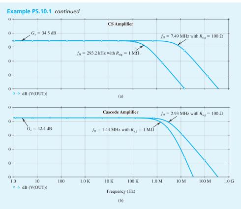
**Figure B.31** Frequency response of (a) the CS amplifier and (b) the folded-cascode amplifier in Example PS.10.1, with  $R_{\text{sig}} = 100 \Omega$  and  $R_{\text{sig}} = 1 \text{ M}\Omega$ .
