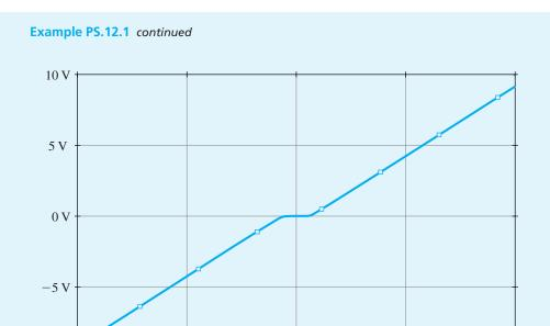
Figure B.41 Transfer characteristic of the class B output stage of Fig. B.37.
