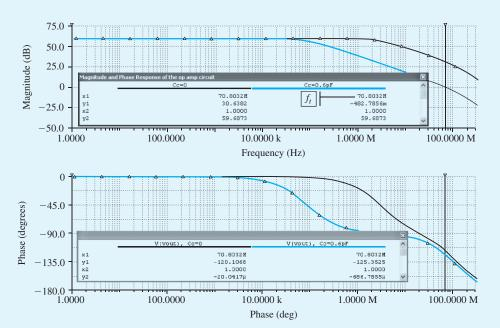
Figure B.109 Magnitude and phase response of the op-amp circuit with R=1.53 k,  $C_{c}=0$  (no frequency compensation), and  $C_C = 1.8 \text{ pF} (PM = 75^{\circ}).$
