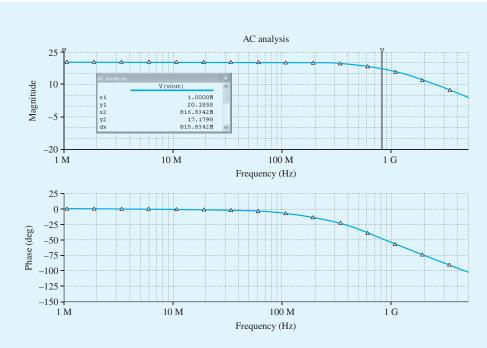
Figure B.101 Frequency response of the closed-loop circuit.
