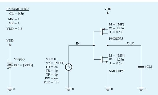
Figure B.49 Schematic capture of the CMOS inverter in Example PS.14.1.
