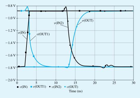
**Figure B.58** Transient response of a cascade of two ECL gates interconnected by a 1.5-m coaxial cable having a characteristic impedance of  $50 \Omega$  and a delay of 10 ns (see Fig. B.57).
