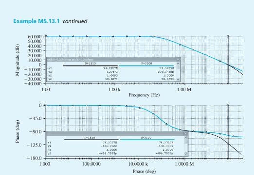
**Figure B.111** Magnitude and phase response of the op-amp circuit with  $C_c = 0.6$  pF, R = 1.53 k $\Omega$  ( $PM = 55^{\circ}$ ), and R = 3.2 k $\Omega$  ( $PM = 75^{\circ}$ ).
