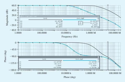
Figure B.110 Magnitude and phase response of the op-amp circuit with  $R = 1.53 \text{ k}\Omega$ ,  $C_C = 0$  (no frequency compensation), and  $C_C = 1.8 \text{ pF} (PM = 75^{\circ}).$
