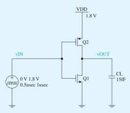
Figure B.114 Schematic capture of the CMOS inverter.
