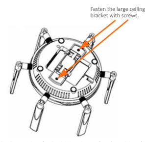
2 Supporting the SonicWave in one hand, position the edge clips of the bracket over the edge of the ceiling crossbar and rotate the SonicWave counterclockwise (to the left when looking up at it) until the bracket is securely attached to the crossbar.
