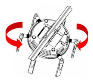
To remove the SonicWave 432e or SonicWave 432i from the ceiling crossbar, rotate it *clockwise* (to the right when looking up at it) until the bracket detaches from the crossbar.
