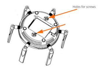
To mount the SonicWave 432e or SonicWave 432i to a crossbar between ceiling panels using the large bracket:
