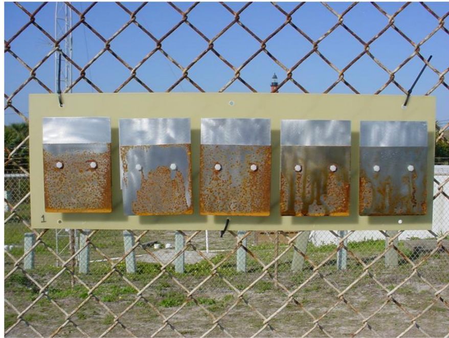
Lap Splice Coupon Sets Mounted on Chain Link Fence at FMRF
