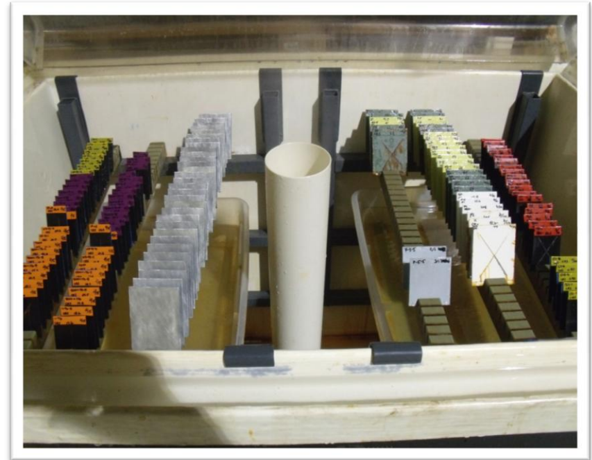
UC samples in salt fog chamber at ECOSIL
