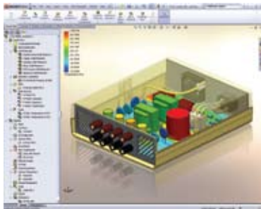
Simulate electronic design with multiphysics for fluid flow as well as thermal analysis.
