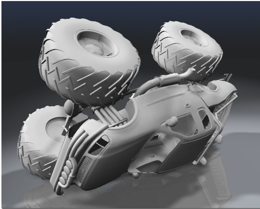
Figure 1: Using particles with orientation enables us to simulate a complex model like this monster truck with plastically deforming body, free spinning wheels with soft tires, and high fidelity mesh skinning in real time all with a sparse physical representation.
