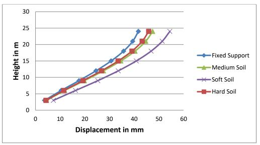
Fig 4.18: Comparison of Displacement v/s Height for Five Storey Building with rectangular footing
