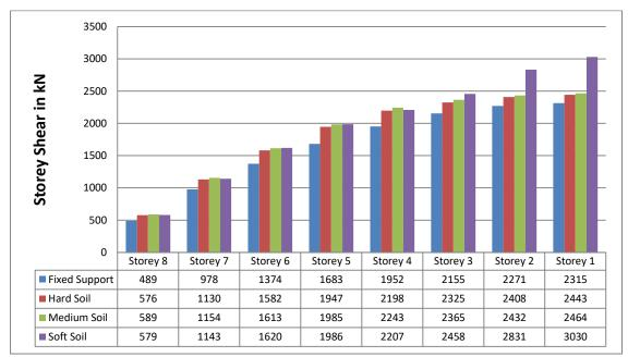
Fig 4.14: Variation of Base Shear for Eight Storey with square footing
