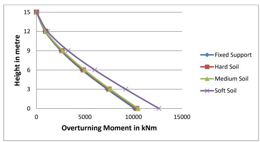
Fig 4.21: Overturning Moment v/s Height for five Storey building with Square footing
