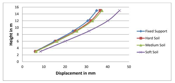
Fig 4.17: Comparison of Displacement v/s Height for Five Storey Building with square footing
