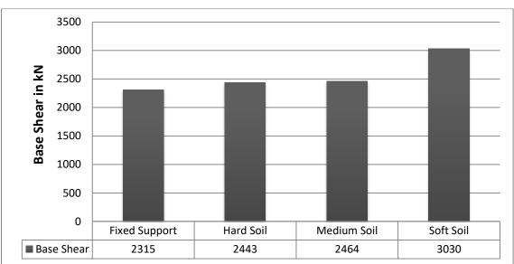
Fig 4.15: Variation of Storey Shear for Eight Storey with Rectagular footing
