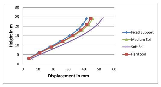
Fig 4.20: Comparison of Displacement v/s Height for Eight Storey Building with rectagular footing
