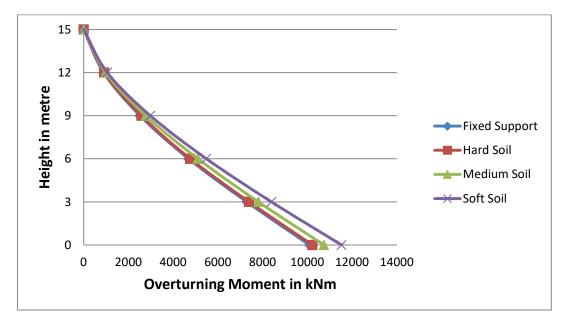
Fig 4.22: Overturning Moment v/s Height for Five Storey Building with Rectagular footing
