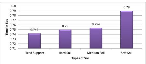
Fig 4.6: Variation of Twisting Time Period for Eight Storey Building supported on Square Footing
