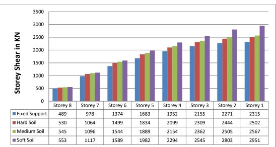
Fig 4.12: Variation of Base Shear for Five Storey building with Recatagular Footing
