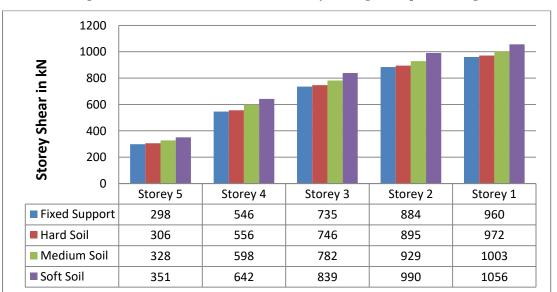
Fig 4.10: Variation of Base Shear for Five Storey building with Square Footing
