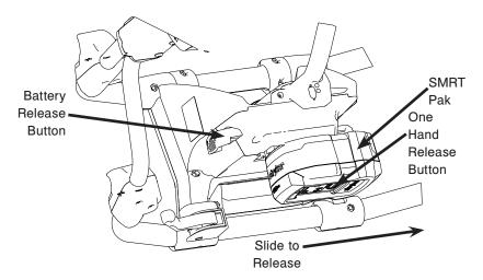
Figure 9: SMRT Pak Removal and Replacement
