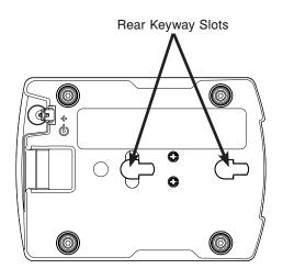
Figure 3: Charger Rear Keyway Slots
