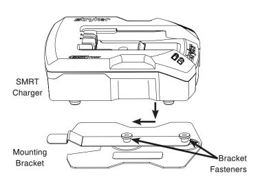
Figure 4: Installing the Charger
