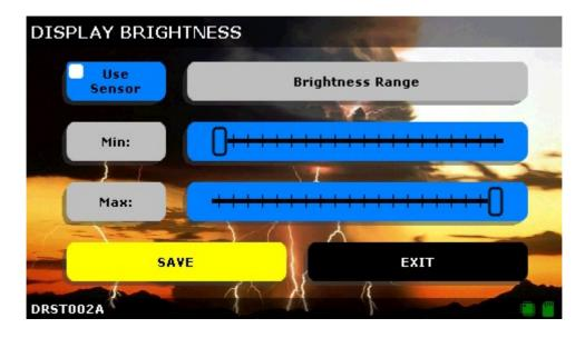
On this part of the menu you can do a few things. The most useful being the "Use Sensor" Option. The monitor has a sensor in the front that will detect the current light level, and adjust the brightness accordingly.
