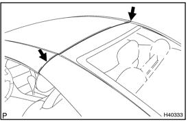
Strongly push down the roof panel and the back window near the parting line.
