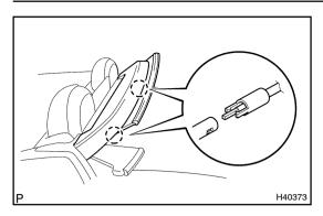
(b) Disconnect the joints of the cables from the package tray trim gear box.
