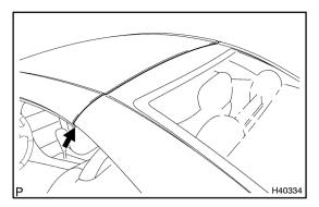
Push up the roof panel and the back window near the parting line and check that they are locked.
