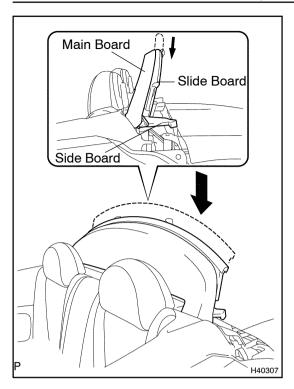
(d) Place both your hands on the slide board in the positions close to both ends and push it down.
