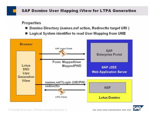
Figure 7: Application of SAP User Mapping to authenticate to Domino and to generate the Ltpa Token
