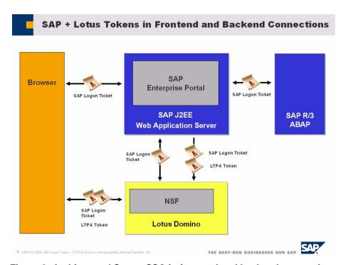
Figure 3: Architectural Setup: SSO in frontend and backend connections
