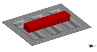
Simulates Plasticomp CF35 PA6 Charge size:138 mm, 27.8 mm, 27.5 mm
