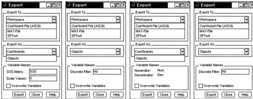
(a) To save a SOS filter structure as a variable or a filter object (b) To save filter coefficient(s) as a variable or a filter object
