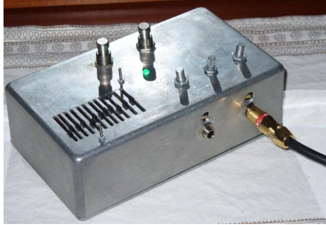
Figure 29: Input and output jacks mounted to the box, the LED is green which indicates that the distortion block is switched on and the equalizer block is in bypass.
