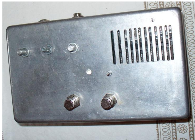
Figure 30: LED indicator light is not lit even though the bypass switches have not been adjusted since the previous picture, because the input cable has been removed from the pedal removing power from the circuit.
