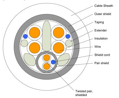
Figure 10: Cross section of the integrated cable with two encoder cables
