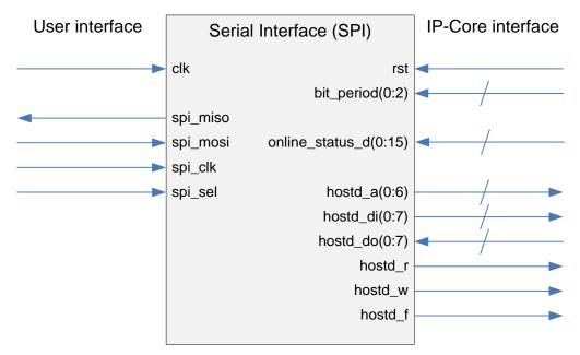
Figure 38: Serial interface block signals
