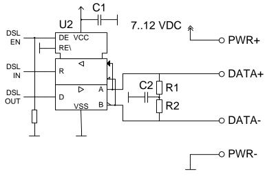
Figure 5: Interface circuit with separate encoder cable
