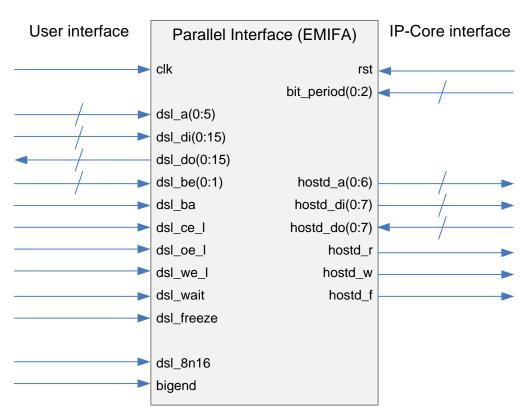
Figure 40: Parallel interface block signals
