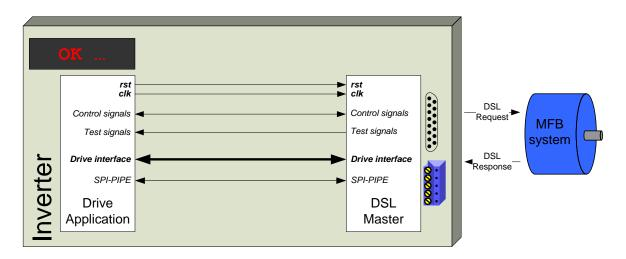
Figure 11: DSL system interfaces
