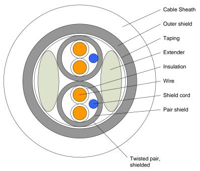
Figure 9: Cross section of the separate encoder cable with four encoder cables
