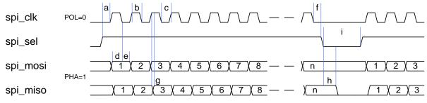
Figure 39: Time control of the SPI
