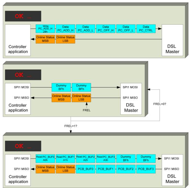
Figure 30: Example of a "long message" read command
