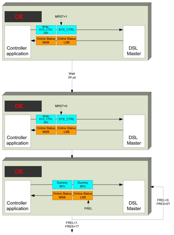
Figure 31: Reset of the Parameters Channel
