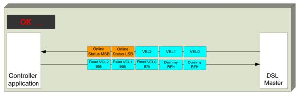
Figure 23: Polling of rotation speed registers in free running mode
