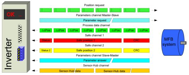
Figure 3: Data channels in HIPERFACE DSL<sup>®</sup>
