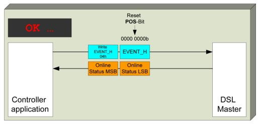
Figure 32: Acknowledgment of event bits
