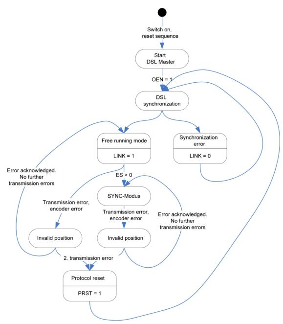
Figure 20: Status table for DSL system start.
