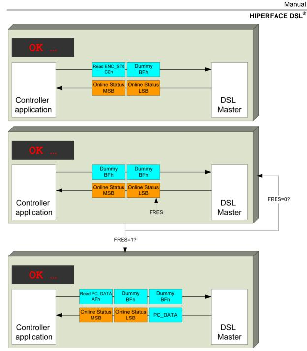
Figure 28: Reading from remote register
