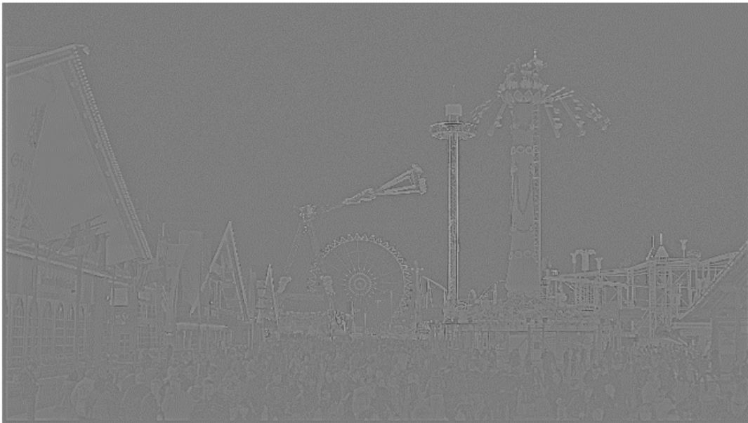
Figure 6 - Enlarged View of the Spatial Detail Signal for the Luma Component
