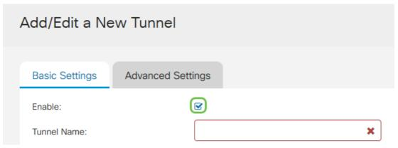
Step 4. Enter a name for the VPN connection in the Tunnel Name field.
