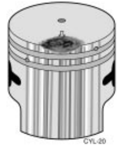
Figure 2.6 Damage caused by preignition.
