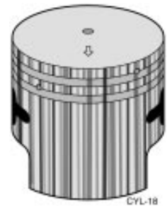
Figure 2.3 Piston damaged from lack of lubrication.
