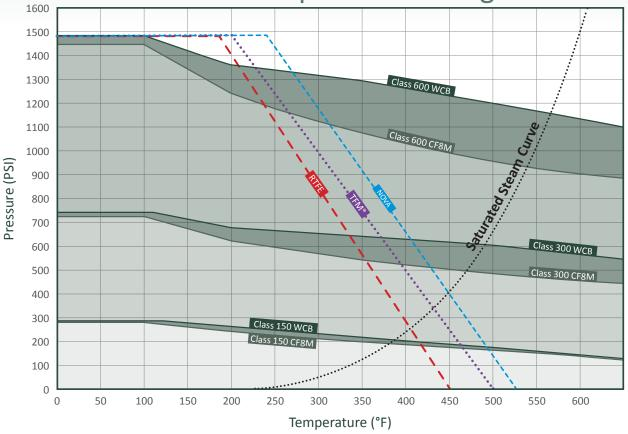
The maximum pressure/temperature ratings of the valve assemblies are limited to lowest of the body or seat material fitted.
