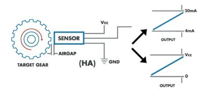
Target: Ferrous Material Gear Tooth with range of Min. 4 to 32 Gear Pitch  $P = \frac{N+2}{OD} \begin{vmatrix} P = \text{Gear Pitch} \\ N = \text{Num. of Teeth} \\ OD = \text{Outside Diameter} \end{vmatrix}$ Frequency: 15 kHz Max
