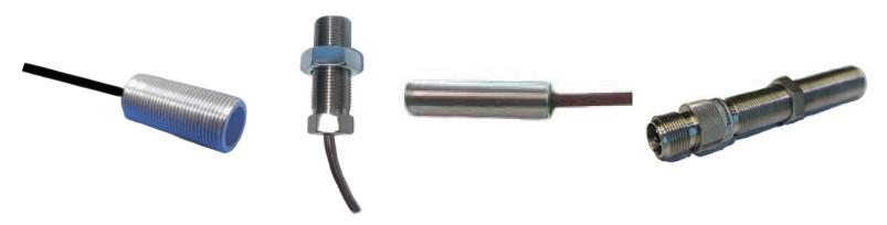
Non-contact magnetic sensor proximity switch produces a digital output. The output produced by Hall-Effect Proximity Switch sensor switches between logic low (operate point) and logic high (release point) with presence and absence of a magnet as a target. The built-in hysteresis circuitry allows clean switching of the output even in the presence of external mechanical vibration and electrical noise.
