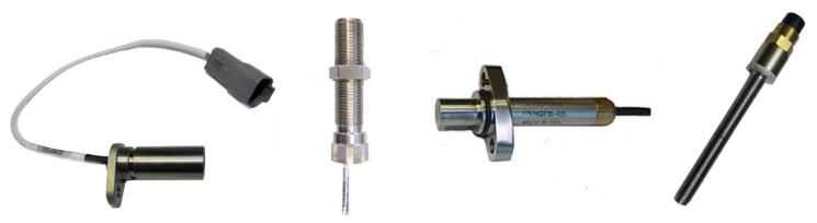
Non-contact magnetic sensors that measure the distortion of magnetic field created by a ferrous target. Quadrature sensors provide two 90° out of phase digital outputs to record speed and direction. When the target wheel or gear is rotating clockwise, the output signal # 1 leads output signal # 2, and when the target is rotating counter clockwise, the output signal # 2 leads output signal # 1. Both output signals will be 50% duty cycle with proper alignment of sensor and target gear.
