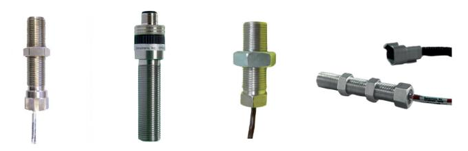
Non-contact linear speed magnetic sensors that uses Hall effect technology to measure the velocity of a rotating object. This sensor is a complex device with signal conditioning that is powered and provides a 4 - 20 mA or a 0 - 10 VDC linear output for velocity measurement.
