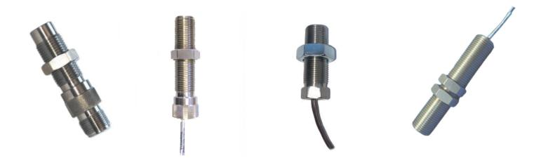
Due to the active solid state signal conditioning integral with this variable reluctance speed sensor, it converts a sine wave signal output to produce a digital square wave signal with constant amplitude regardless of variations in speed.
