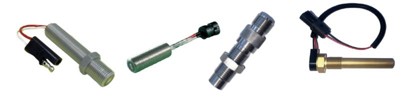
The collapse of magnetic field due to the interruption by a ferrous gear tooth provides an analog signal output (sine wave) that does not require an outside power source. Variable reluctance sensor or Mag-pickup is suitable for speed sensing with a range from 30 to 1000 inches per second with a target gear from one tooth per revolution to 32 pitch gear.
