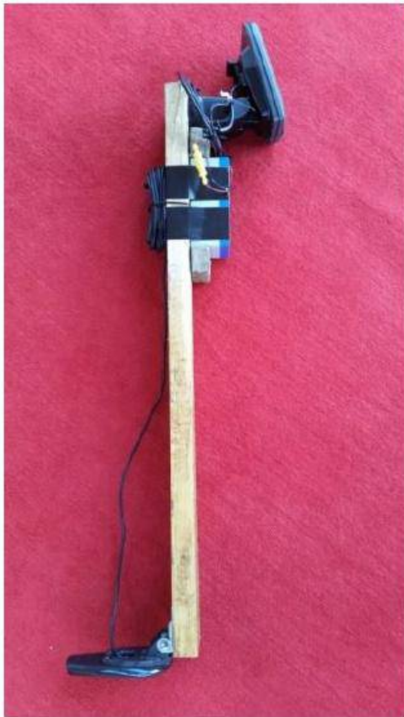
Figure 31: the echo sounder setup
