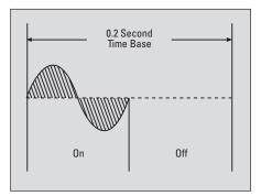
Figure 1. Time-proportioned, zero-cross burst.
