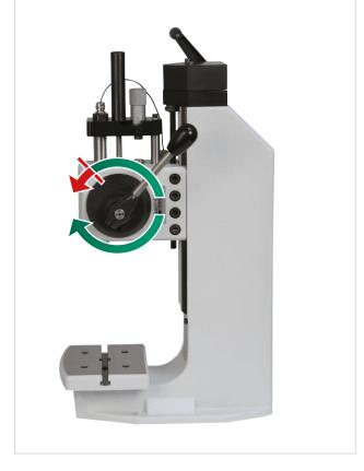
Forward Stroke Lock Mode (the return Stroke is released) For protecting the produced parts and the force sensor of the press the press blocked/restricts the force flow in forward stroke when reaching a defined force or when reaching the stroke.
