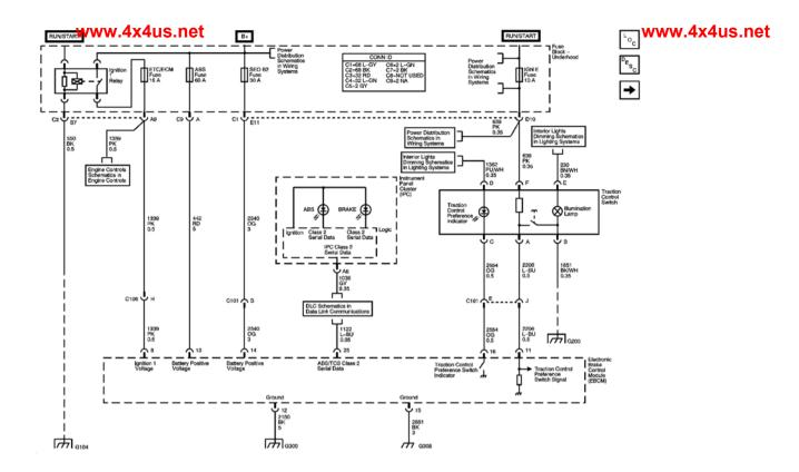
Fig. 1: EBCM Power, Ground, DLC, Indicator Lamps, and Traction Control Switch Courtesy of GENERAL MOTORS CORP.
