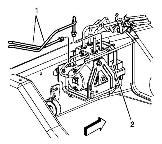
www.4x4us.net Fig. 11: Rear Brake Pipes & BPMV Courtesy of GENERAL MOTORS CORP.
