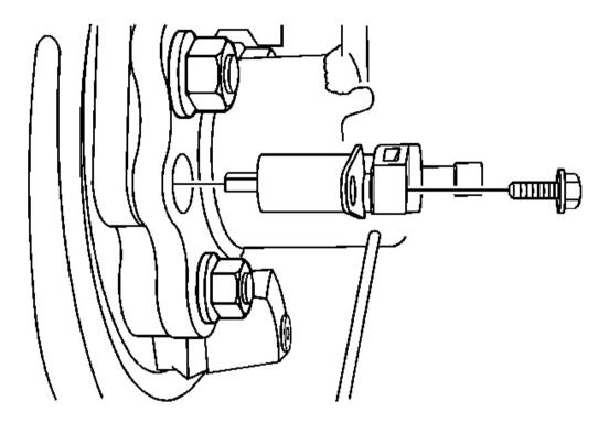
Fig. 18: Rear Wheel Speed Sensor & Shim Courtesy of GENERAL MOTORS CORP.
