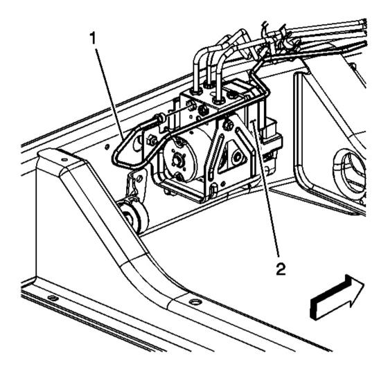
**Fig. 7: Right Front Brake Pipe & BPMV** Courtesy of GENERAL MOTORS CORP.
