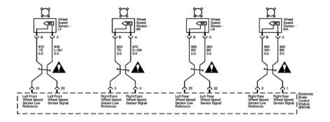
**Fig. 3: Wheel Speed Sensor Inputs** Courtesy of GENERAL MOTORS CORP.
