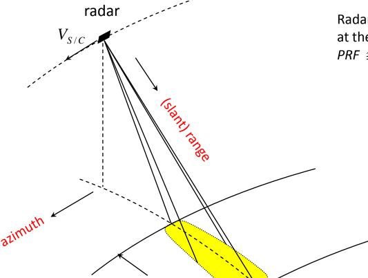
Radar transmits pulses and receives echoes at the rate of the pulse repetition frequency:  $PRF \cong 1000 - 4000 \text{ Hz}$
