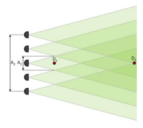
Length of synthetic aperture depending on distance between antenna and target
