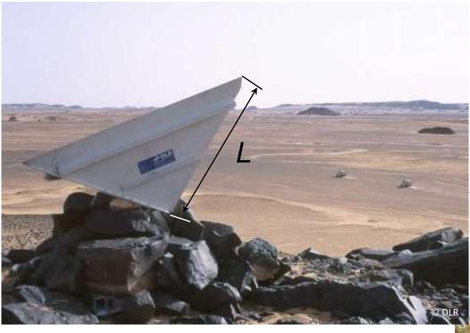
radar cross section of a trihedral corner reflector:
