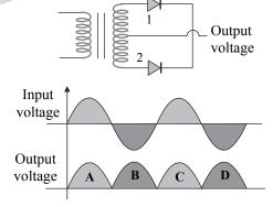
The contribution to output voltage from diode 2 is
