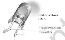
A diode which finds extensive u. in rolling displays, traffic some use it system etc. A light emittin dio cc emit light of a particula lou. nen fe ward biased.
