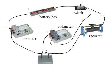
A student wants to measure the resistance of a resistor R and sets up the circuit shown. The student made which of these mistakes setting up the circuit ?
