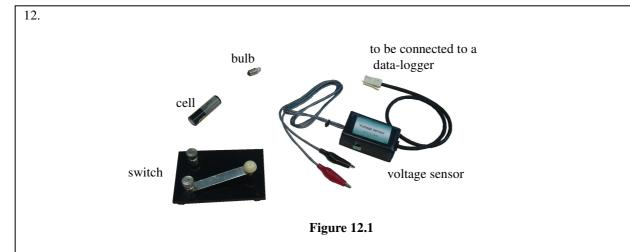
Iris uses the apparatus shown in Figure 12.1 to study the lifetime of AA-size cells when used to power a bulb. She connects a cell and a switch to the bulb and uses a voltage sensor to measure the voltage across the bulb.
