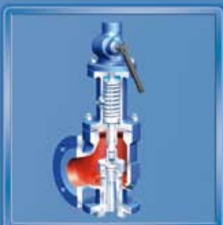
SAFE-FN ANSI acc. to API526 closed lifting device
