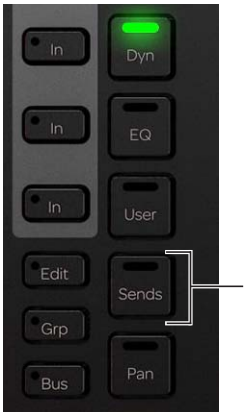
Sends switch on the Process Module
