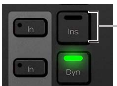
Inserts switch on Process Module
