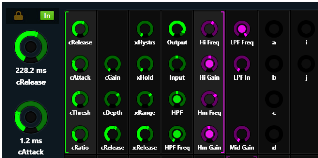
Figure 53. Function Editor with brackets indicating which parameters are assigned to left (green) and right (purple) Attention Track Knobs
