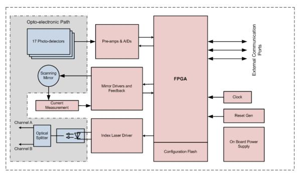
Figure 5: OMM block diagram
