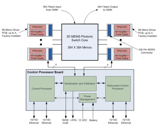
Figure 3: MSM320 block diagram
