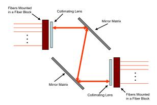
Figure 2: Light path within the MSM320
