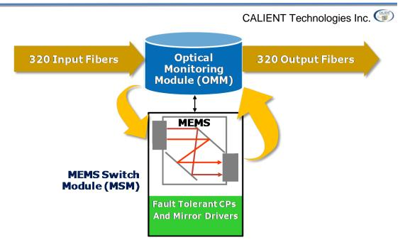
Figure 1: CALIENT S320 Photonic Switch Architecture
