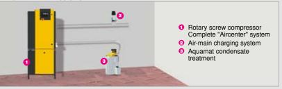
Only properly designed air systems can meet the demands for air quality, availability and efficiency that are placed on a modern compressed air supply. Therefore benefit from decades of compressed air engineering experience and let KAESER design your compressed air supply system.
