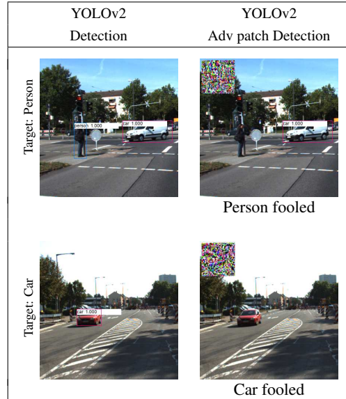
Figure 3: Evaluation on KITTI dataset - Examples of trained universal patch for car and person.
