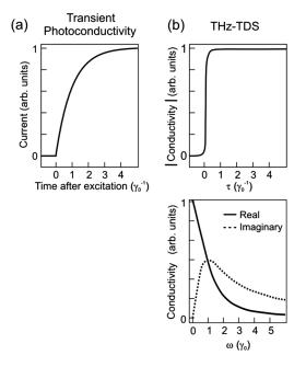
FIG. 5. Time dependence of signals in a (a) transient photoconductivity measurement and (b) THz-TDS measurement, both for a Drude electron gas undergoing a step increase in density at time zero.
