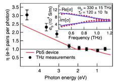
FIG. 6 (color online). Number of generated electron-hole pairs per photon in bulk PbS ( $E_{gap} = 0.42 \text{ eV}$ ) as a function of photon energy (circles). Also shown is the results of a device measurement (sloping solid line) from Smith and Dutton (1958). The inset shows the conductivity and the fit to the Drude model and corresponding plasma frequency and scattering time. From Pijpers *et al.* (2009).
