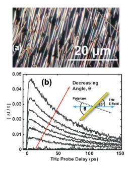
FIG. 24 (color online). (a) Dark-field optical micrograph of oriented germanium nanowires. (b) Measured differential transmission for various polarizer angles  $\Theta$ . Inset: Sketch of the geometry of nanowire orientation, THz electric field, and polarizer angle  $\Theta$ . From Strait *et al.* (2009).
