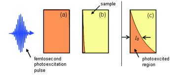
FIG. 2 (color online). Schematic of typical sample excitations achieved in an optical pump-THz probe experiment. Experiments with (a) homogeneous excitation and (b) interfacial excitation can be treated analytically.
