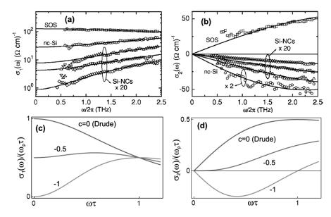
FIG. 20. (a) Real part and (b) imaginary part of the conductivities of photoexcited charge carriers in bulk and nanocrystalline silicon; the lower panels show exemplary plots of the Drude-Smith model for various values of c: (c) real conductivity; (d) imaginary conductivity—both vs frequencies normalized to  $\omega\tau$ . From Cooke *et al.* (2006).
