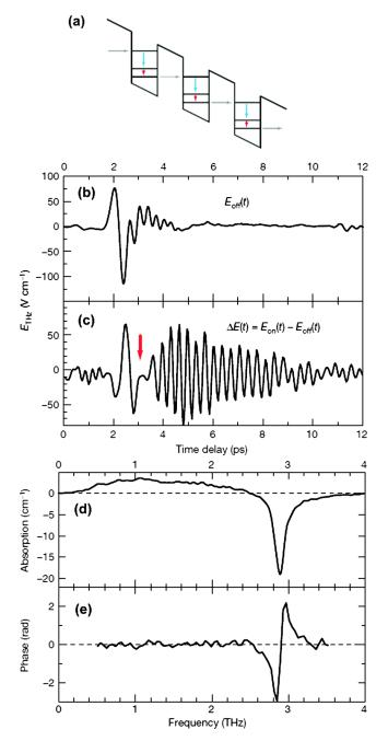
FIG. 30 (color online). Terahertz time-domain spectroscopy of a THz quantum-cascade laser: (a) Schematic of a quantum-cascade laser; (b) THz probe transmitted through an unbiased QCL; (c) change in the transmitted probe through a biased QCL; (d) absorption spectra, and (e) phase of the bias-modulated probe. From Kroll, Dhillon *et al.* (2007).
