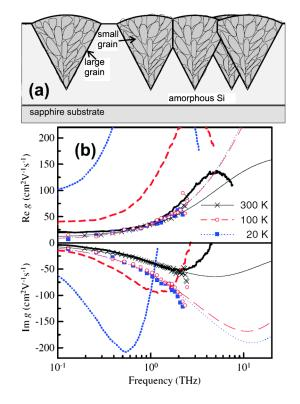
FIG. 21 (color online). (a) Scheme of the composition of the microcrystalline samples under investigation by Fekete *et al.* (2009), (b) Mobility spectra of charge carriers in microcrystalline silicon for temperatures of 300, 100, and 20 K at a pump-probe delay of 50 ps. Upper panel: real part, lower panel: imaginary part. Symbols: experimental data, thick lines: Monte Carlo simulations incorporating backscattering, thin lines: fits to hopping model. From Fekete *et al.* (2009).
