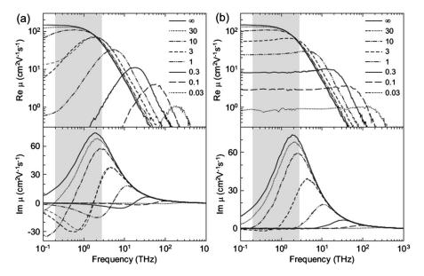
FIG. 26. Mobility spectra of localized particles calculated by Monte Carlo simulations for various values of  $\alpha$  (upper panels: real part, lower panels: imaginary part). (a)  $p_r = 1$ , (b)  $p_r = 0.5$ . From Nemec, Kuzel, and Sundstrom (2009).
