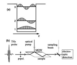
FIG. 27. (a) Sketch of the electron wave functions in subbands of quantum wells; (b) schematic of a optical pump-THz probe experiment on multiple-quantum-wells samples. From Golde *et al.* (2009) and Luo, Reimann, Woerner, Elsaesser *et al.* (2004).
