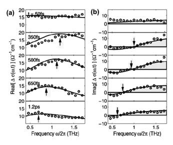
FIG. 23. (a) Real part and (b) imaginary part of the conductivity of photoexcited charge carriers in GaAs nanowires for various pumpprobe delays. A redshift of the localized surface plasmon resonance frequency is observed (indicated by the arrows): trapping at surface states decreases the charge carrier density over time and hence the plasmon frequency. From Parkinson *et al.* (2007).
