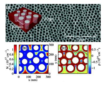
FIG. 25 (color online). (a) Scanning electron micrograph of the surface of nanoporous InP; the inset shows a three-dimensional cartoon of the porres. Simulations of the spatial distribution of the carrier density in nanoporous InP at 100 K: (b) Before photo-excitation regions close to the pores are depleted of charge carriers due to band bending. (c) After photoexcitation, the bands flatten out and charge carriers are distributed more homogenously. From Lloyd-Hughes *et al.* (2008).
