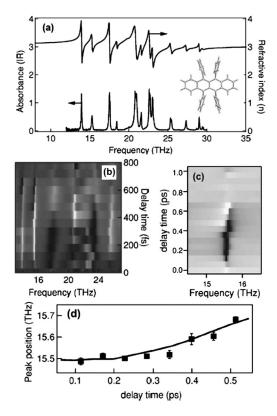
FIG. 15. (a) Linear absorption spectrum and refractive index of a rubrene crystal; the inset shows its molecular structure; (b) frequency-resolved real part of the transmission change  $\Delta E/E$  as a function of pump-probe delay; (c) close-up of the transmission change of the resonance around 15.5 THz; (d) experimental (squares) and modeled (solid line) shift of the resonance frequency vs pump-probe delay. From Koeberg *et al.* (2007).
