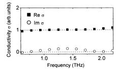
FIG. 8. Conductivity of an organic crystal pentacene at room temperature; the dashed lines are guides to the eye for a flat, frequency-independent response. From Ostroverkhova *et al.* (2005).
