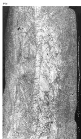
Figure 27: Thin-section through interface shear zone sampled from clay 'cake' adhering to ICP tested at Pentre, showing system of multiple oriented 'residual' shear surfaces 11
