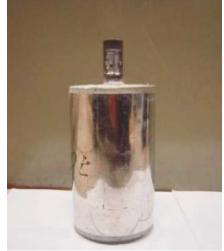
Completed Steel Jacket
