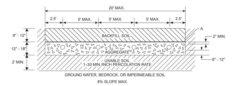
FIGURE 18: DISTRIBUTION LATERAL SPACING FOR ABSORPTION TRENCH OR BED
