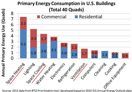
Figure 1-1: Building primary energy consumption by end-use
