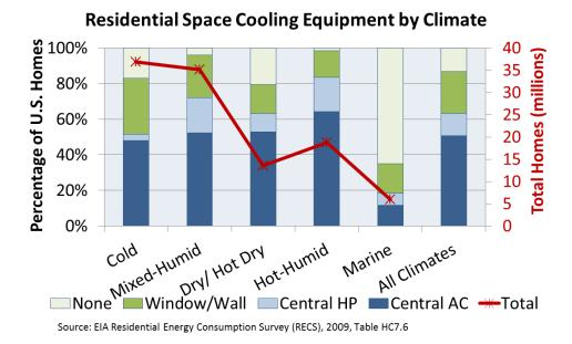
Figure 3-2: Residential space cooling equipment by climate
