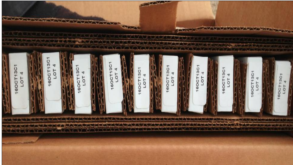
Photo 4: Packing Instruction 1 Intermediate Packaging (Fiberboard Dividers)
