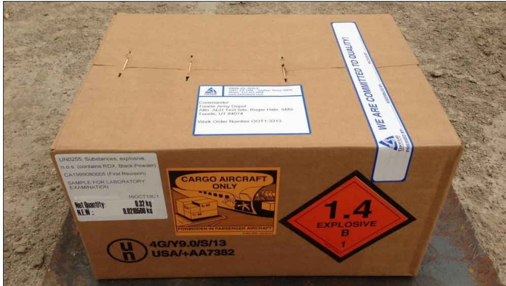
Photo 2: Packing Instruction 2 Outer Packaging (4G Fiberboard Box)
