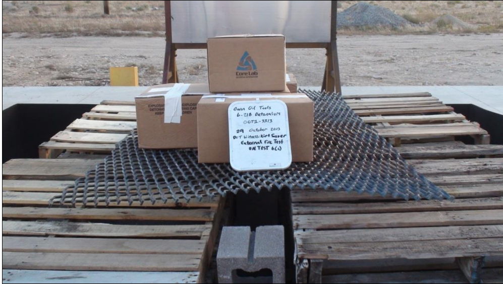
Photo 9: External Fire Test Setup
