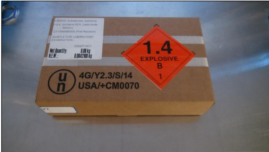
Photo 2: Packing Instruction 1 Outer Packaging (4G Fiberboard Box)
