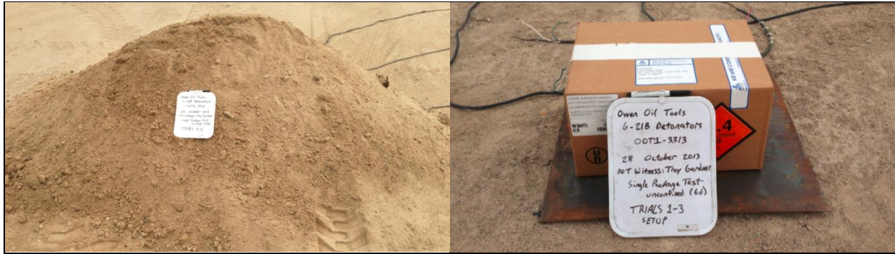
Photo 7: Single Package Test Setup, Confined (left) and Unconfined (right)
