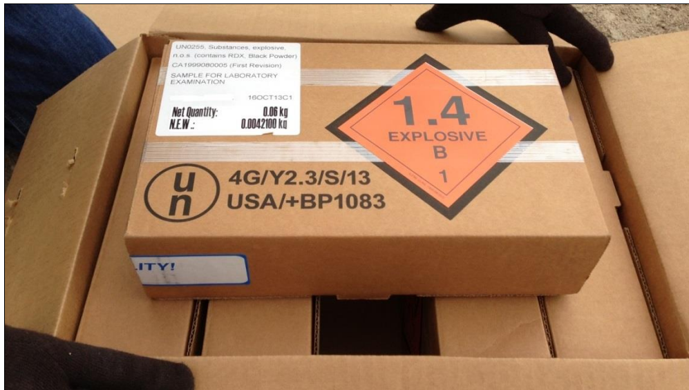
Photo 3: Packing Instruction 1 Outer Packaging (4G Fiberboard Box)
