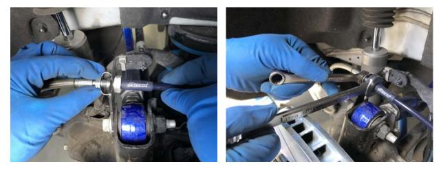
**NOTE:** Double check the **UPPER** stainless line clearance to ensure there is neither excessive binding tension, nor interference with any suspension components. Make necessary adjustment by re-clocking the 90° swivel male-end fitting to reposition.
