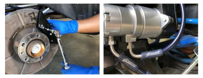
Determine the  $\bigcirc$  UPPER stainless line's angle of rotation by inserting temporarily the inboard end of the UPPER stainless steel brake line fitting through the existing hole of the locating bracket (as image shown). Once the position is confirmed, use an 11mm wrench to tighten the 90° swivel male-end fitting to 14 ft/lbs (19n/m).
