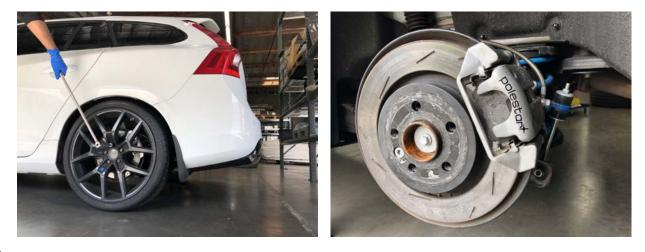
WARNING: Rotora recommends setting the vehicle to SERVICE (MAINTENANCE) MODE prior to the removal of the entire rear OEM brake system so that the Electronic Parking Brake (EPB) system can retract back to full release position. This procedure varies depending on the vehicle model and the diagnostic scanning software tool.
