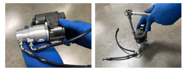
NOTE: Ensure that the orientation of the servomotor to the new LEFT-SIDE EPBB module is as image shown.
