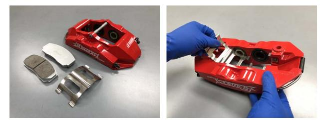
Insert one brake pad into position on one side of the caliper by setting the pad spring clip into tension. Then insert another brake pad onto the other side to set the spring clip into full tension. Ensure that the friction side of each brake pad is facing the brake disc.
