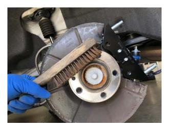
Mount the new LEFT-SIDE disc/hat assembly, ensuring that it is seated firmly on the hub face. Reinsert the original disc retaining set screw with a T-50 TORX Impact Driver/bit socket.
