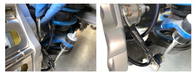
NOTE: Do not use a torque wrench, as over tightening the bolt can strip the aluminum threads, causing irreparable damage to the caliper.
