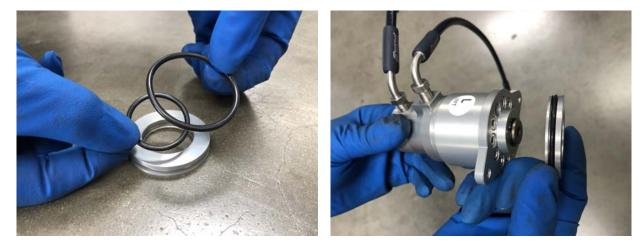
Using a T30 TORX bit, attach the original servomotor to the new EPBB module with the original 2 retaining screws.
