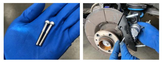
NOTE: Ensure that the orientation of the new LEFT-SIDE EPBB-servomotor assembly to the mounting bracket is positioned as image shown.
