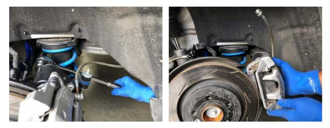
Remove the disc retaining set screw with a T-50 TORX Impact Driver/bit socket (retain this screw for later use) and remove the original brake disc.
