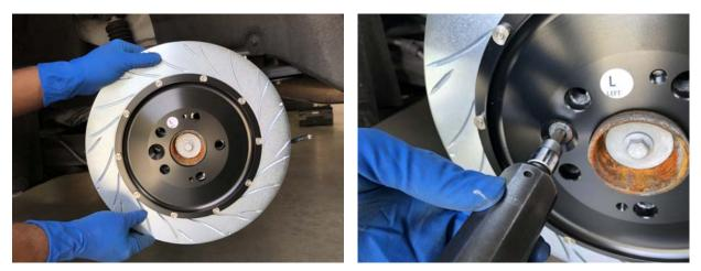
NOTE: Make sure the new disc is on the correct side of the vehicle. Reversing the discs will severely decrease the cooling capacity of the system. Refer to diagram on page 1 to determine direction.
