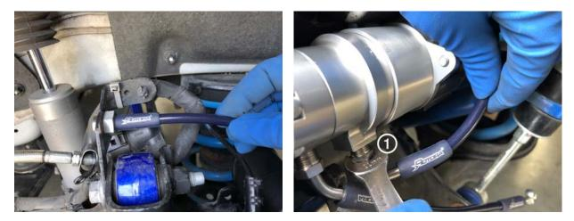
Determine the ② LOWER LEFT-SIDE stainless line's angle of rotation by presetting the Banjo fitting end to where the caliper inlet port location will be (as image shown below). You may temporarily mount the Rotora caliper onto the new bracket to determine the actual rotating angle. Once the position is confirmed, use an 11mm wrench to tighten the 135° swivel male-end fitting to **14 ft/lbs (19n/m)**.
