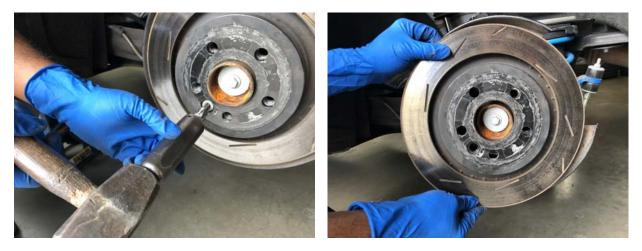
NOTE: It may be necessary to strike the brake disc on the outer edges with a rubber mallet if corrosion prevents the disc from coming off. If so, place a wheel lug in one of the holes first, to prevent the disc from falling when it comes loose.
