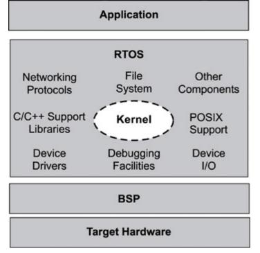
Figure 4.1: High-level view of an RTOS, its kernel, and other components found in embedded systems.
