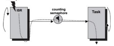
Figure 15.10: ISR-to-task synchronization using counting semaphores.
