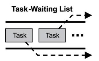
Figure 8.14: Condition variable control block.
