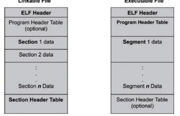
Figure 2.4: Executable and linking format.
