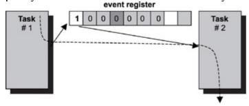
Figure 15.8: Task-to-task synchronization using event registers.
