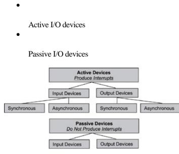
Figure 14.4: Some general properties of active and passive devices.
