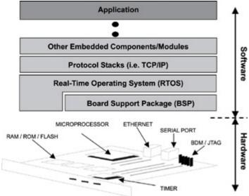
Figure 3.6: Software components of a target image.
