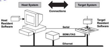
Figure 2.1: Typical cross-platform development environment.
