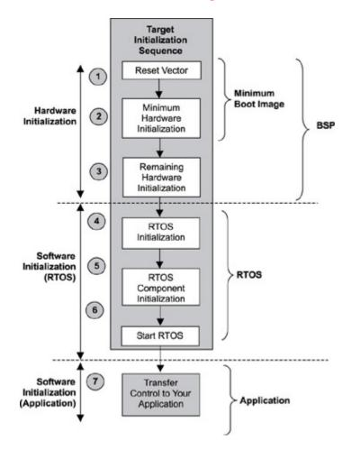
Figure 3.7: The software initialization process.
