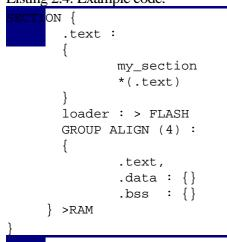
The SECTION command in the linker command file instructs the linker to combine the input section named my\_section and the default .text sections from all object files into the final output .text section. The loader section is placed into flash memory. The sections .text, .data, and .bss are grouped together and allocated in contiguous physical RAM memory aligned on the 4-byte boundary, as shown in Figure 2.7. Executable Image
