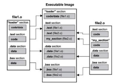
Figure 2.6: Combining input sections into an executable image. Listing 2.4: Example code.
