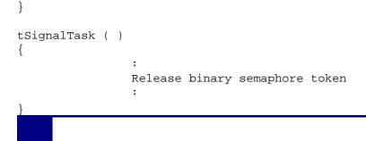
Because tWaitTask's priority is higher than tSignalTask's priority, as soon as the semaphore is released, tWaitTask preempts tSignalTask and starts to execute.
