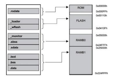
Figure 2.8: Mapping an executable image into the target system.
