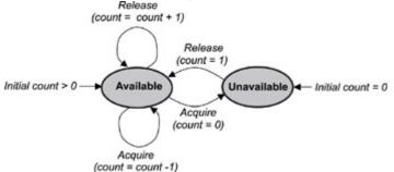
Figure 6.3: The state diagram of a counting semaphore.
