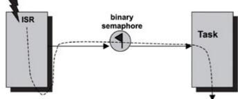
Figure 15.7: ISR-to-task synchronization using binary semaphores.
