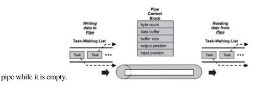
Figure 8.3: Pipe control block.
