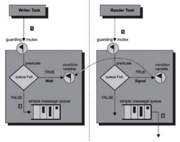
Figure 15.20: Using condition variables for task synchronization.
