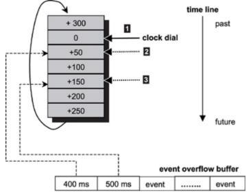
Figure 11.14: Timing wheel overflow event buffer.
