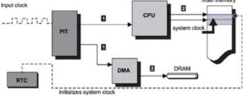
Figure 11.2: System clock initialization.
