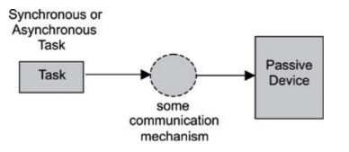
Figure 14.6: General communication mechanisms for passive I/O devices.
