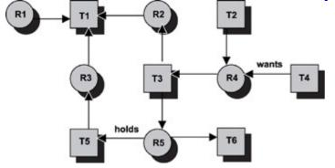
Figure 16.5: Deadlock eliminated by proper resource reassignment.
