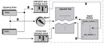
Figure 15.21: Using signals for urgent data communication.
