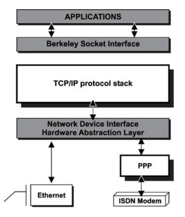
Figure 9.2: TCP/IP protocol stack component.
