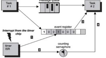
Figure 15.19: Task with multiple input communication channels.
