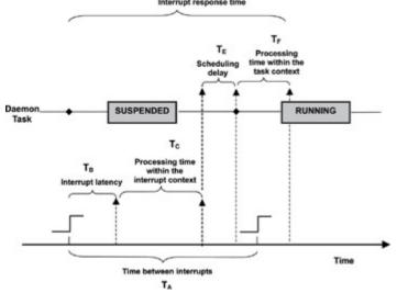
Figure 10.10: Interrupt processing in two contexts.
