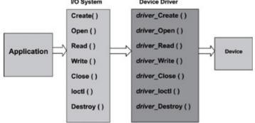
Figure 12.6: I/O function mapping.
