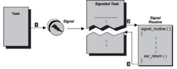
Figure 15.12: Using signals for urgent data communication.
