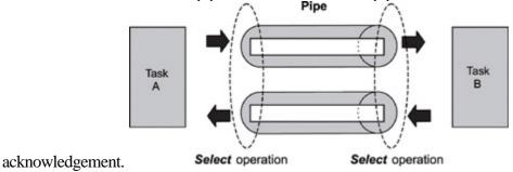
Figure 8.6: Using pipes for inter-task synchronization.
