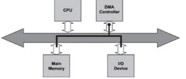
Figure 12.4: DMA I/O.
