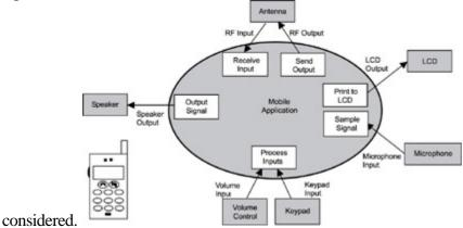
Figure 14.2: Using the outside-in approach to decompose an application into tasks.
