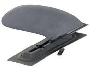
Turn the kayak over and slide the skeg into the base. It only slides in facing one way. Slide the locking tab into its groove until it clicks into place.
