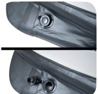
Side drains are intended to drain accumulated water while ashore. Leaving the drains opened while on the water will cause water to enter the kayak. Keep drains closed while kayak is in use. If drains leak, refer to Troubleshooting.
