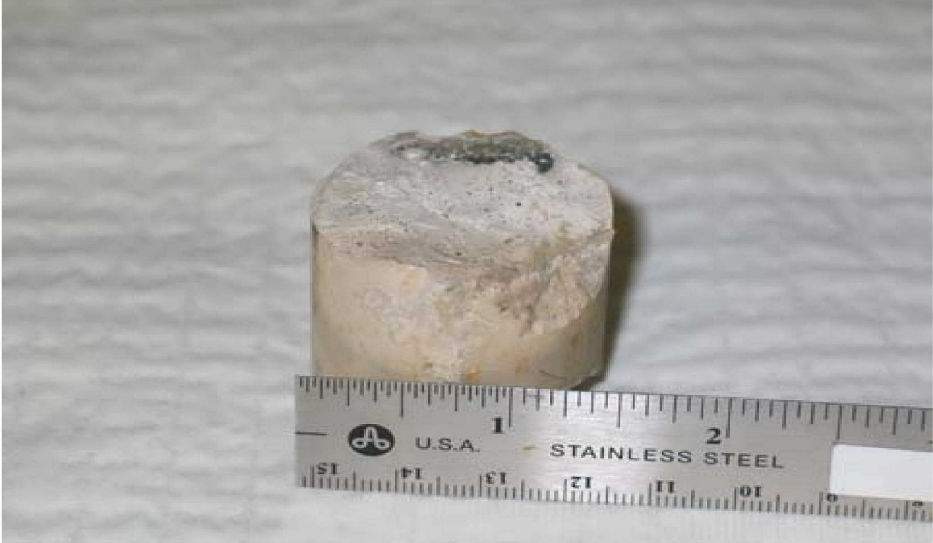
Figure 4. Test cylinder generated using slag/sand mixtures
