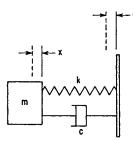
**FIGURE 2.20** Single degree-of-freedom system with viscous damper, excited in forced vibration by foundation motion.
