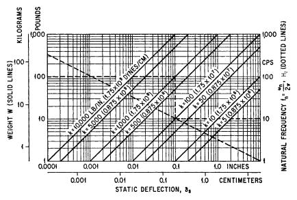
where W = mg is the weight of the rigid body forming the mass of the system shown in Fig. 2.4. The relations of Eq. (2.8) are shown by the solid lines in Fig. 2.5.
