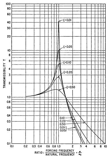
FIGURE 2.17 Transmissibility of a viscous-damped system. Force transmissibility and motion transmissibility are identical numerically. The fraction of critical damping is denoted by  $\zeta$ .
