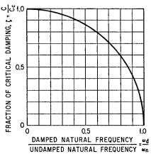
FIGURE 2.7 Damped natural frequency as a
