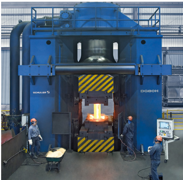
Counterblow hammer with 800 kJ working capacity.
