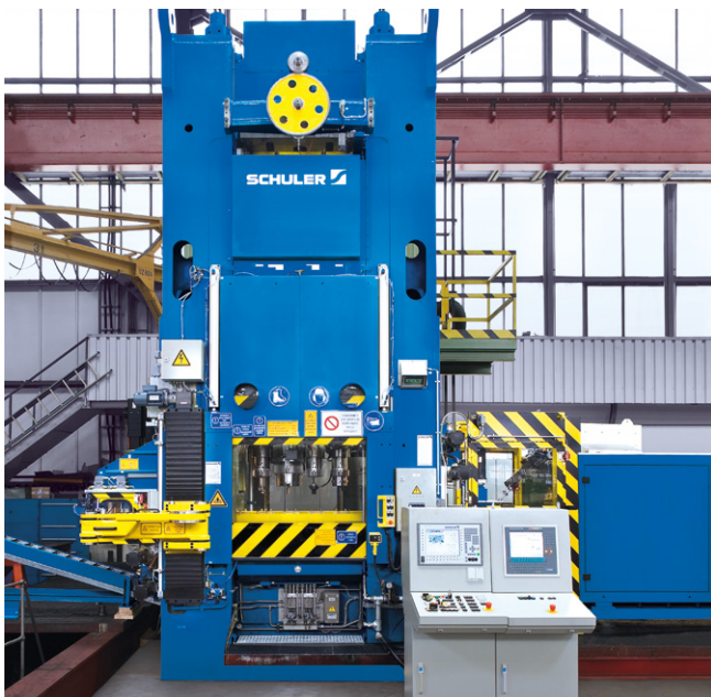
The mechanical press is the main component of the complete system for manufacturing sleeper screws.
