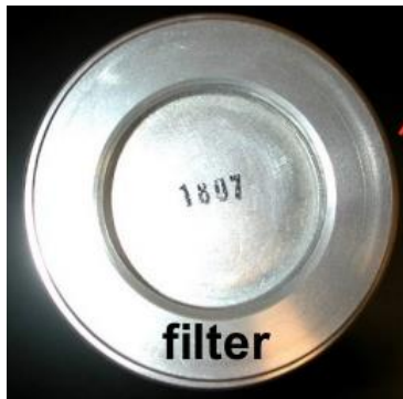
fig 3: aluminum filter attached to the tube head
