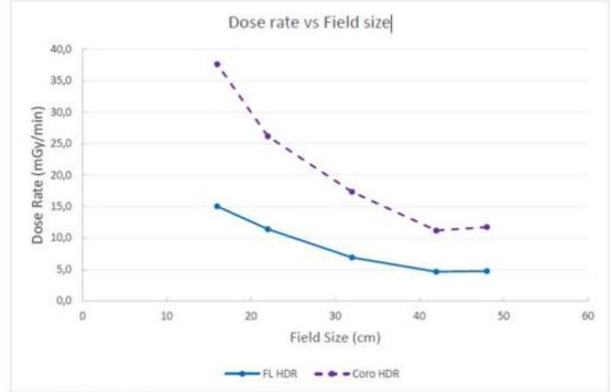
Figure IV. This graph shows how the dose rate (measured at the table) varies as a function of the field size for FL HDR and Coro HDR. As expected the dose rate drops with increasing field size and the fluoroscopy program lies well below the acquisition one.
