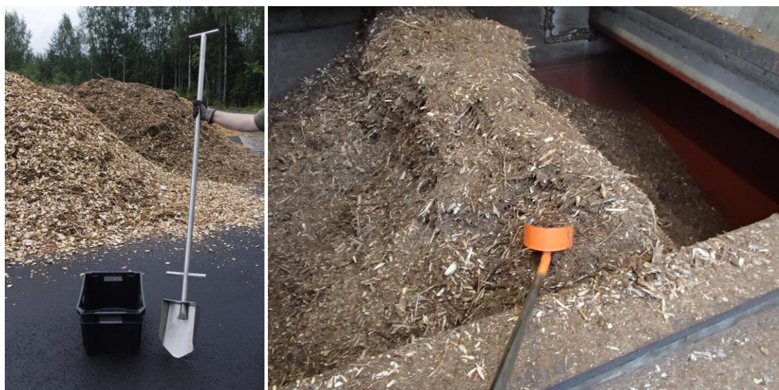
Figure 2. Pictured (on the left) a shovel-type sampler for collecting samples from a fuel stockpile and on the right, a three-litre sampling scoop for collecting samples from a moving stream. Photos: Haklog ky and Ismo Tiihonen.
