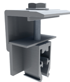
Image 2.4.9 Universal end clamp [96 in-lbs (11 N-m)]
