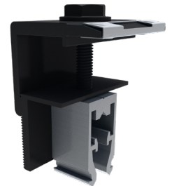
Image 2.4.10-1 Universal end clamp w/WEEB-BMC [96 in-lbs (11 N-m)]
