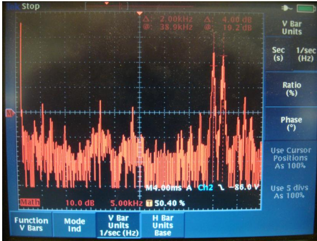
Figure 58: Unfiltered Output FFT w/200W Resistive Load
