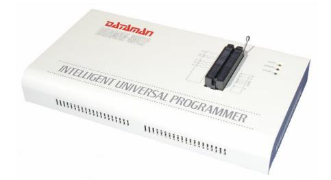
Place your PIC microcontroller in the black ZIF socket and place the silver lever in the down position to clamp onto the I/O pins.
